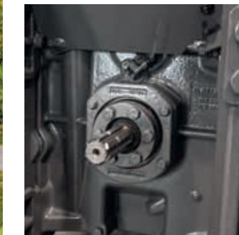
The Fendt Vario CVT provides a simple, proven design that eliminates wear components such as clutch packs. The PTO rotates independently of the transmission.
