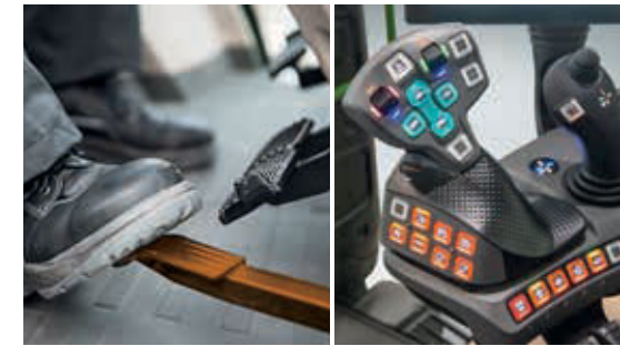
Driving pedal or joystick control: The driving mode can be selected individually. The speed can be controlled with either the pedal or the joystick. Change drive direction either with the joystick or the reverse lever with built-in stop and go function.
