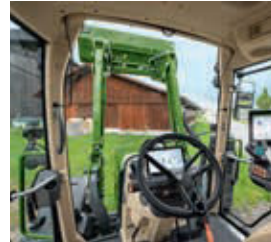
Panoramic front window with 77° vision for a full view upwards and over the wheel arches.
