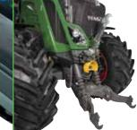
Optional factory installed front PTO, 3-point, and hydraulic valves make this the most multi-purpose tractor available
