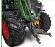
Standard 40-GPM hydraulic system with optional 54-GPM independent hydraulic pump with up to 6 rear and 2 front hydraulic valves; single and double acting front 3-point options give you the right configuration for any application.
