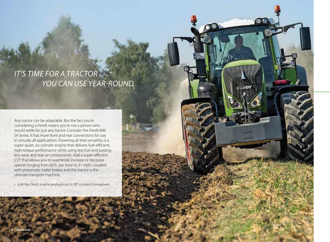
Optional Fendt Stability Control (FSC) takes steering precision, driving stability and braking safety to completely new levels. At speeds above 12.4 mph (20 km/h), FSC locks the front axle suspension cylinders and dampens side-to-side movement to ensure maximum stability during transport. When speeds drop below the FSC threshold, the system automatically disengages to ensure maximum ground contact with all four tires.
