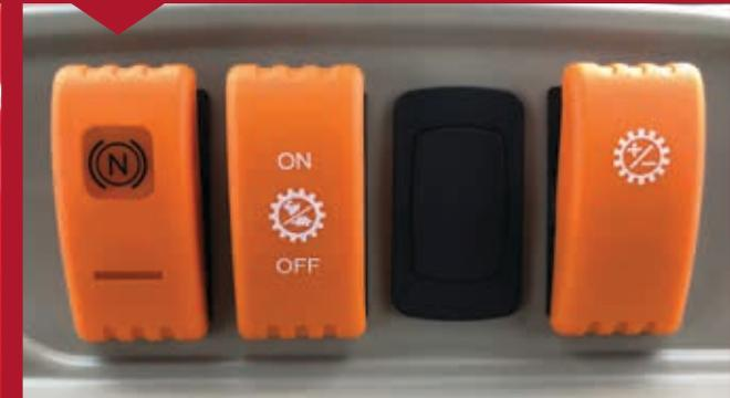
The Speed Matching provides the automatic selection of the appropriate Dyna-2 ratio when a gear change has been made. The speed matching feature minimizes driver effort and maximizes journey times.
