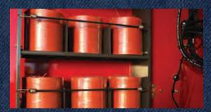
The large twine box adjusts to hold 8 20,000-foot balls or 12 10,000-foot balls, so you can keep baling all day long. The convenient location allows easier access to the baler drives.
