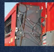
The hydraulically operated main drive clutch protects against overfilling and maintains tension on belts during bale ejection, enhancing belt performance. For quick, easy maintenance, all major drive components are accessed through the convenient one-piece service doors.
