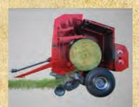
The variable bale chamber design produces a consistently dense bale from the core to the outermost layer. This advanced design delivers a bale that's easy to handle and keeps its shape in storage.
