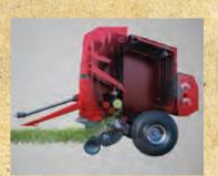
Open-throat feeding assures high-capacity baling on all Hesston round baler models. As the pickup gently moves the hay into the chamber, the forming belts and starter roll begin rolling the all-important bale core.
