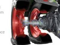
The best warranty in the business — threeyear/3,000-hour full machine warranty, PLUS all scheduled maintenance and a loaner guarantee GOLD STAR CUSTOMER CARE Racecar-influenced, self-leveling front-axle suspension, with 7.8 in. of travel, coupled with a second-to-none pneumatic cab suspension and air-ride seat provides the sophisticated comfort of a luxury pickup truck, even in the field
