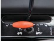
Get extra traction for tough iobs and difficult conditions with on-demand four-wheel drive. Just push the lever downward to engage, pull it up to disengage.
