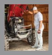
Massey Ferguson takes a wide-open approach to routine maintenance and service. The gas strut makes it easy to raise the hood. Notice how the service points are all easily accessible—and from ground level.
