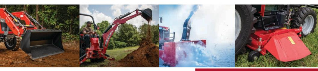
**Start with the FL Series loader.** It's available with a 66- or 72-inch width bucket. The standard skid-steer coupler makes it easy to remove or hook-up the bucket. Add a third remote—and get the versatility of other popular skid-steer attachments—such as a grapple or 4-in-1 bucket.
