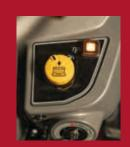
A standard 540-rpm rear PTO and optional 2,000 rpm mid-mount PTO are electrohydraulically controlled for smooth, chatter-free actuation. The smooth SoftStart modulation reduces abrupt jolts, lessens wear and tear and reduces the chance of downtime.
